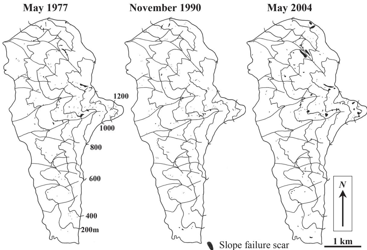
Figure 2: Distribution charts of the slope failures and debris flow scars from the interpretation of aerial photographs
