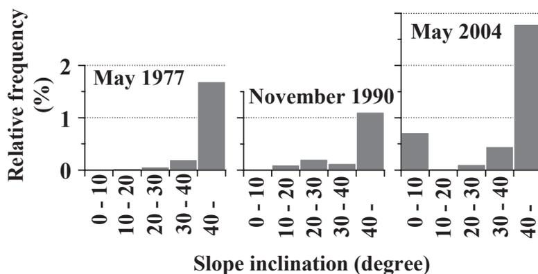
Figure 5: Frequency distributions of the ratio of the areas of slope failures divided into slope inclinations in 10 degree intervals
