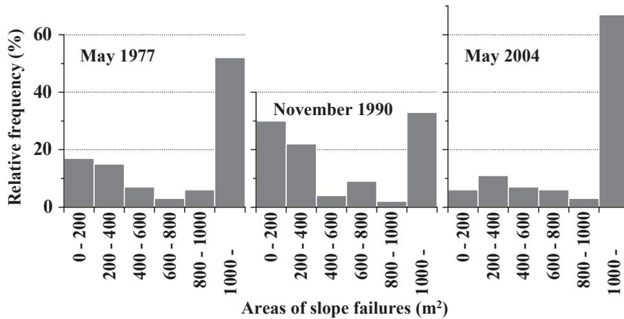
Figure 3: Frequency distributions of the areas of slope failures calculated from distribution charts of the slope failure scars
